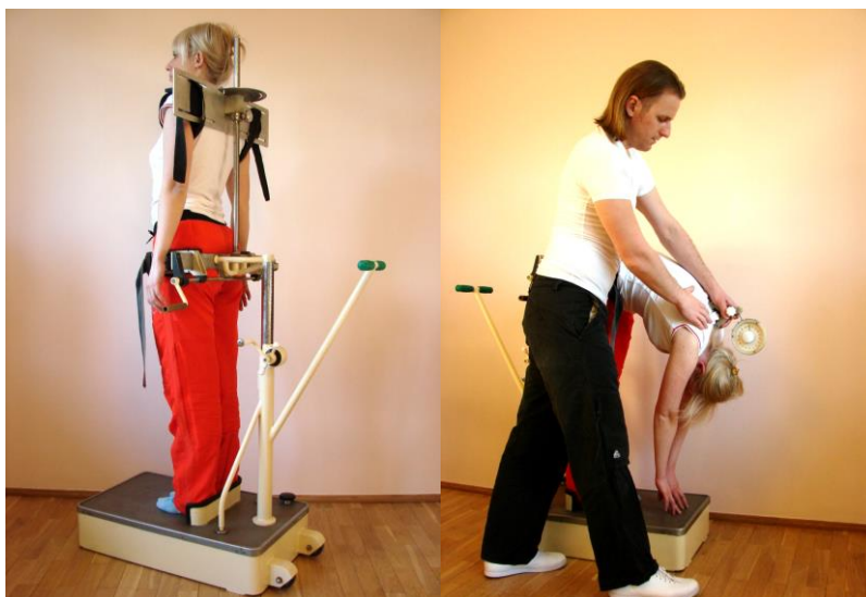
Figure 3 The device invented by prof. Jan Ślężyński for measurements of the spine mobility in sagittal, coronal and transverse planes with pelvis stabilization (patent no. 105042)
